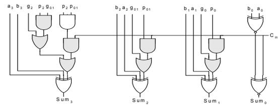
Fig. 3. Four bit area optimized ripple carry adder
