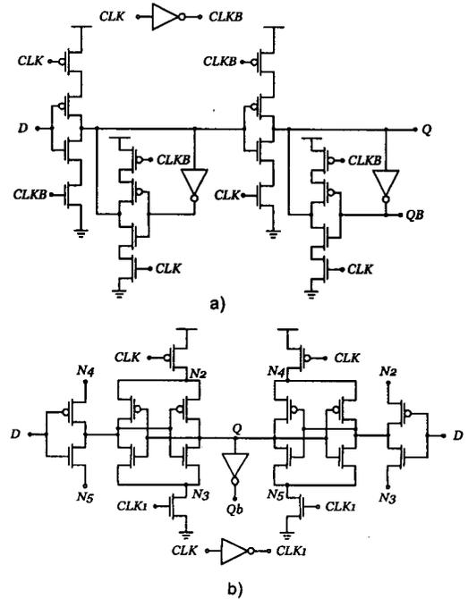
Fig. 3.  $C^2$ MOS a) single-edge master-slave latch and b) double-edge latch-Mux
