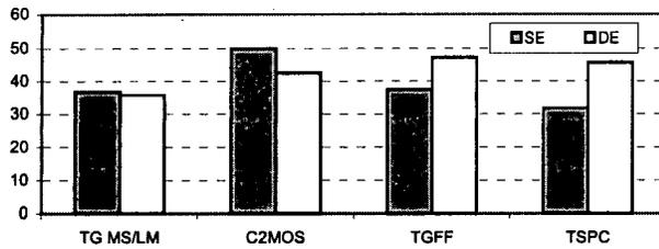
**Fig. 8.** EDP comparison for 50% data activity. EDP in fJ/500MHz for single-edge and fJ/250MHz for double-edge triggered storage elements
