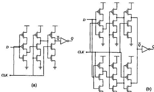
Fig. 5. True Single Phase Clock Latch a) single-edge and b) double-edge version
