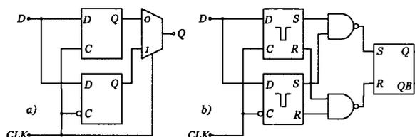
Fig. 1. Basic types of double-edge triggered storage elements a) latch-mux and b) flip-flop
