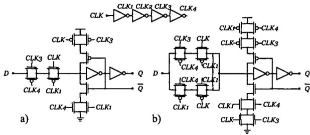
Fig. 4. Transmission Gate Flip-Flop a) single-edge and b) double-edge version
