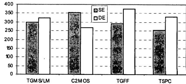
Fig. 7. Delay comparison (time in ps)
