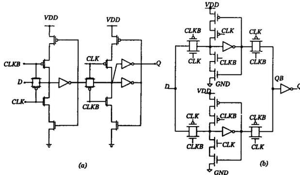
Fig. 2. a) Transmission Gate Master-Slave Latch and b) Transmission Gate Latch-Mux
