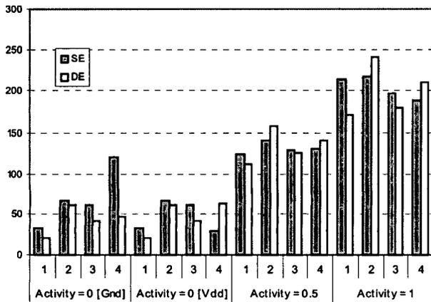
**Fig. 9.** Power consumption vs. data activity (power in  $\mu\text{W}$ ). 1-TGMS/LM, 2- $C^2$ MOS, 3-TGFF, 4-TSPC
