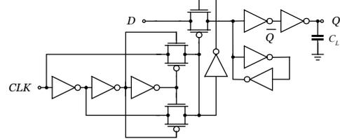
Fig. 3. Explicit-Pulsed Dual Edge Triggered Flip-Flop, ep-DSFF [3]
