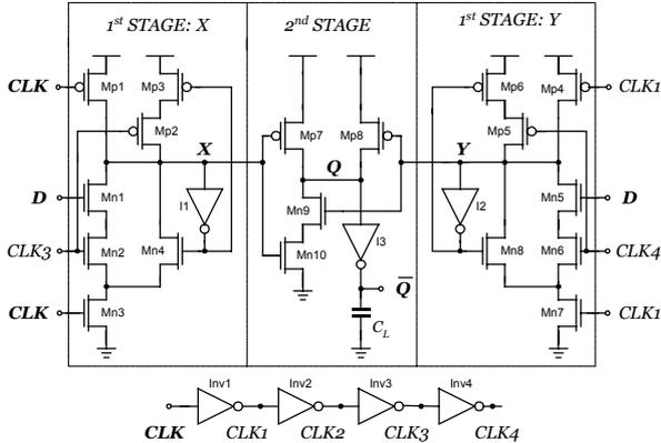
Fig. 1. Symmetric Pulse Generator Flip-Flop, SPG-FF
