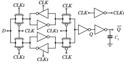
Fig. 4. Transmission-Gate Latch-MUX, TGLM [4]
