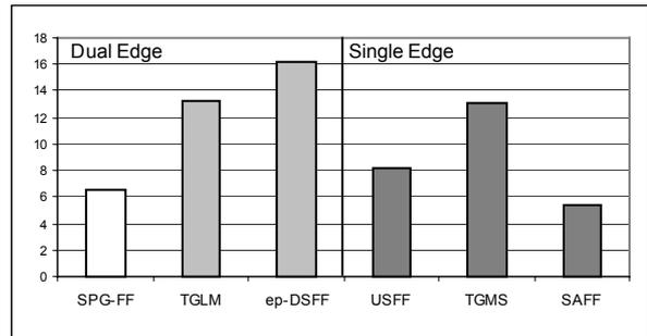
Fig. 7. Comparison of storage elements clock load ( $C_{CLK}$ , load in fF)
