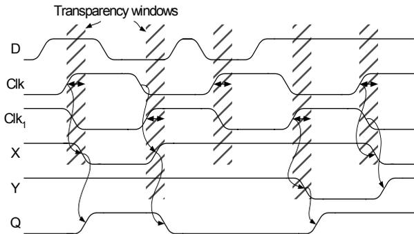
Fig. 2. Timing Diagrams of SPG-FF
