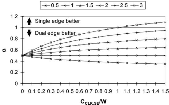
Fig. 9. Dual-edge vs. single edge H-tree power consumption. The parameter is  $C_{CLK,DE}/C_{CLK,SE}$ .
