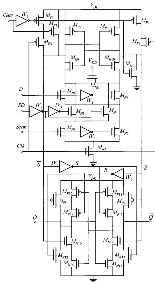
Fig. 8. SAFF with multiplexed scan and asynchronous reset.
