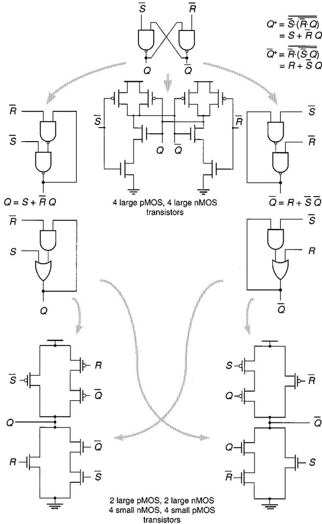
Fig. 4. Steps in obtaining new symmetric SL.
