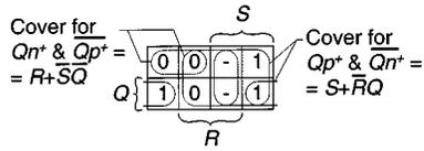
Fig. 3. Karnaugh map for  $Q^+$  and  $\bar{Q}^+$  and equations for resulting pull-up and pull-down transistor networks, labeled as  $Qn^+$  and  $Qp^+$ .
