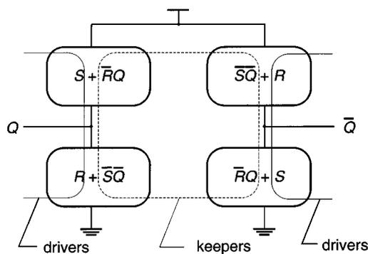
Fig. 7. Transistor functions in the new SL.
