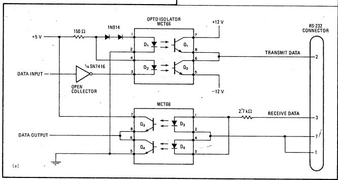
**isolation.** General Instrument's dual-phototransistor opto-isolator MCT66 isolates the RS-232 interface (a) and achieves a high data rate of 9,600 b/s. The signal's polarity may be changed by altering the connections between  $Q_1$  and  $Q_2$  or  $Q_3$  and  $Q_4$  (b).
